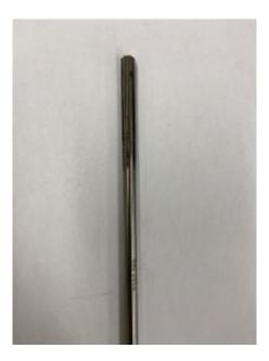
Taps: Taps are used to create threads on the inside of holes. Be aware that there are different types of taps for different operations. Below is a tapered tap (right) and bottoming tap (left). The tapered tap is used to start threads, while the bottoming tap is used to cut threads to the bottoms of holes.
